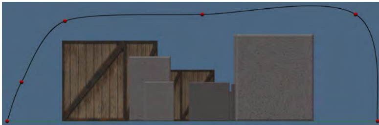
Figure 3.23: Using the elevations map and the previous 2D trajectory we construct the 3D trajectory.
