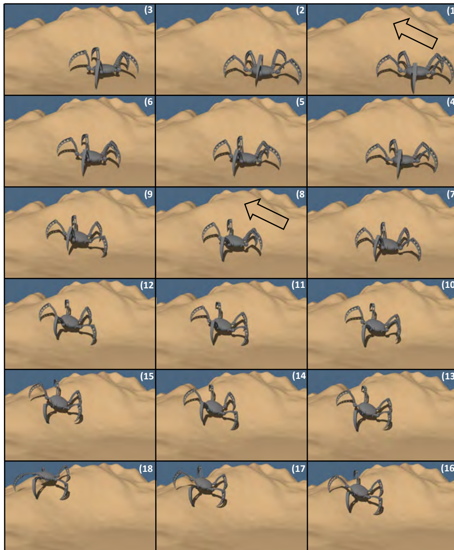
Figure 3.37: A 5-legged robot going uphill.
