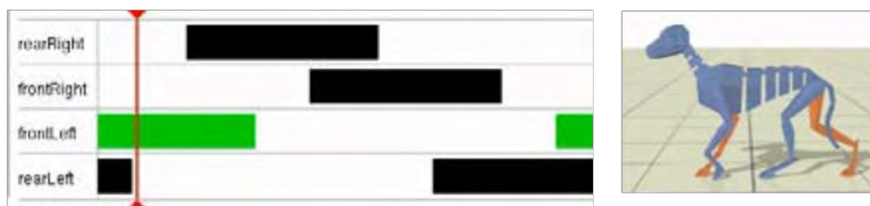
Figure 2.8: Example of a gait pattern: a dog walk cycle, solid bars represent the legs flight phase ( swing phase ), courtesy of [CKJ + 11].
