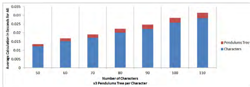
Figure 5.14: Added Calculation time when using pendulums tree in our locomotion system. In seconds.
